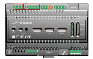
The following table lists the enclosure markings for the RS-232 and RS-485 port screw terminals and on the SmartServer and their connection types.
